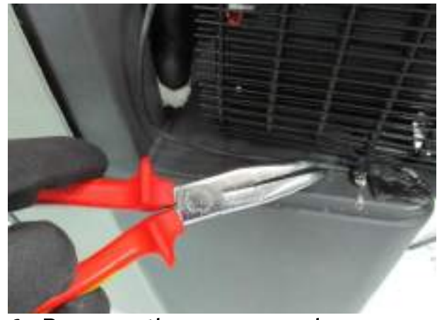
6. Remove the sensor and reverse the procedure to install a new one
