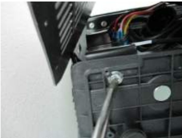
3. Unscrew the bolts (8 bolts)
