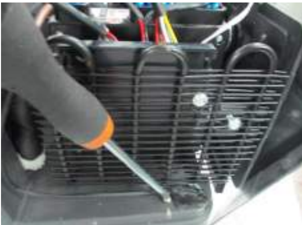
5. Unscrew the bolt that fasten the sensor
