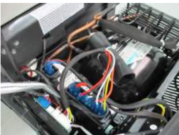
5. Remove the fan's wire
