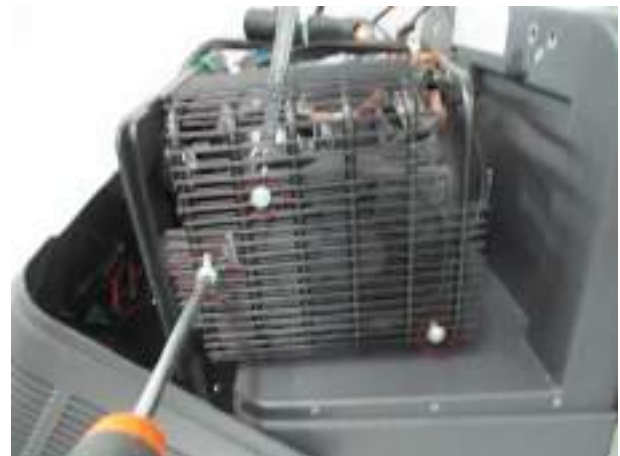
4. Unscrew the bolts from each side (6 bolts)
