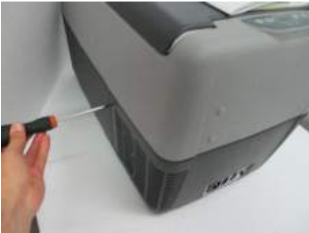
1. Unscrew the plastic support (11 screws)
