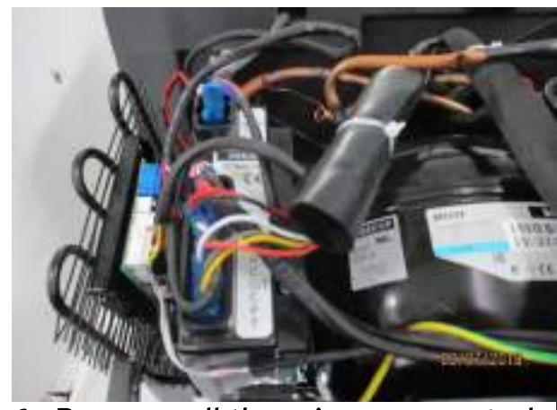
6. Remove all the wires connected to the ECU and then replace the ECU reversing the procedure
